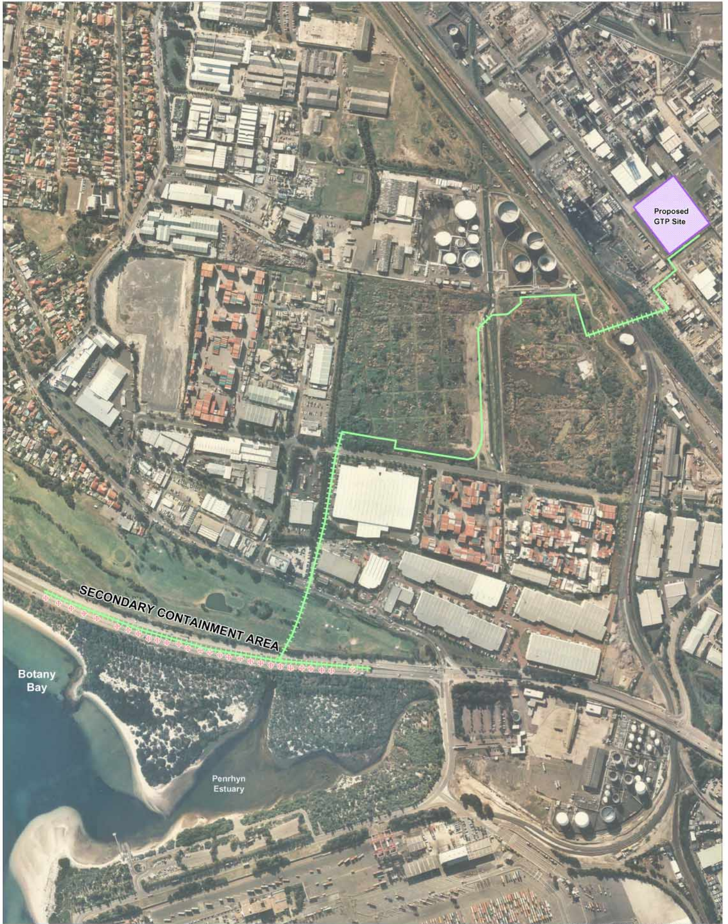
FIGURE 5-7 SCA Groundwater Extraction Wells & Secondary Pipeline
