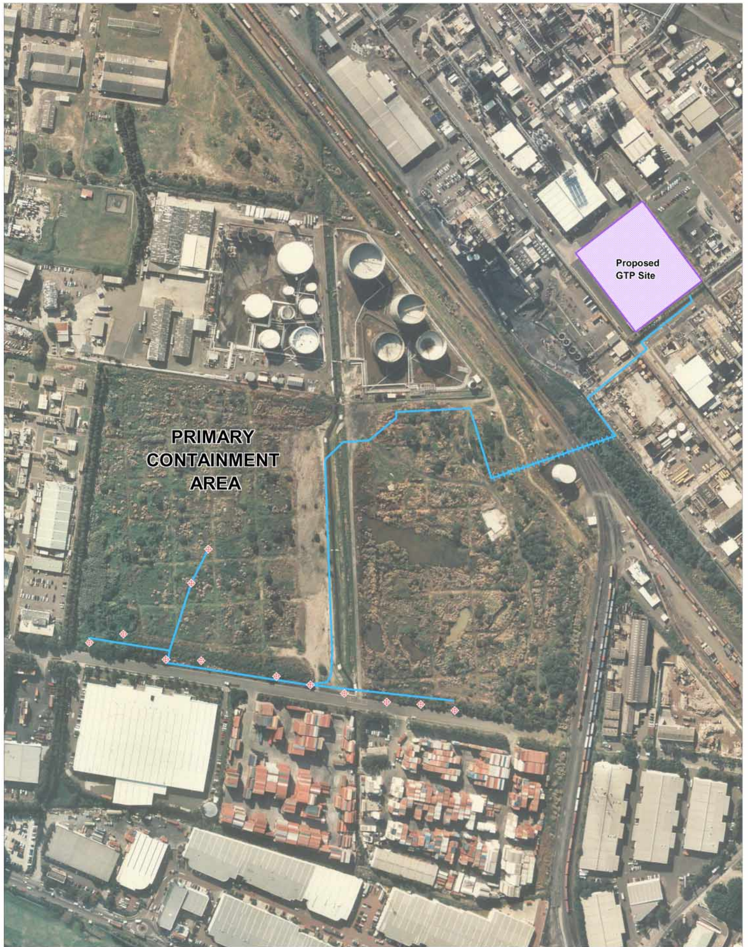
FIGURE 5-3 PCA Groundwater Extraction Wells & Primary Pipeline
