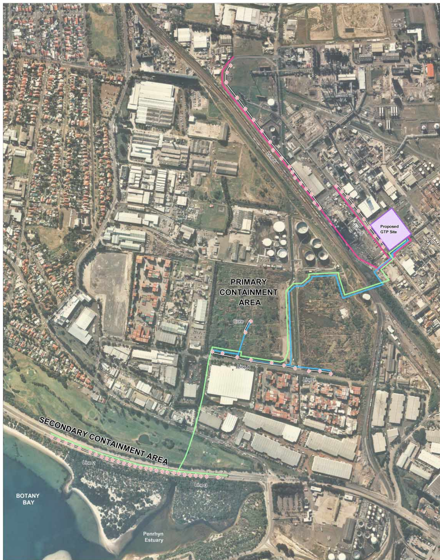
FIGURE 5-2 Groundwater Containment Lines, Extraction Wells & Transfer Pipelines
